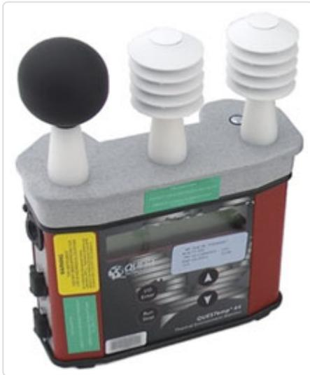
WBGT meters have three sensors that input data into a calculation that adjusts the temperature to represent the impact humidity, wind, and radiant heat have on heat strain cooling effectiveness.
