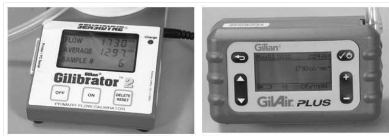
Figure F-6. Gilibrator Display Panel Showing Flow Rate, Side by Side with Gilair Sampling Pump with Digital Flow Readout
