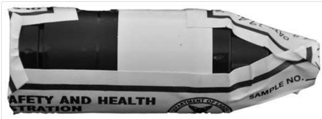
Figure G-5. Standard Asbestos Cassette (25mm) Correctly Sealed With a Form OSHA-21
