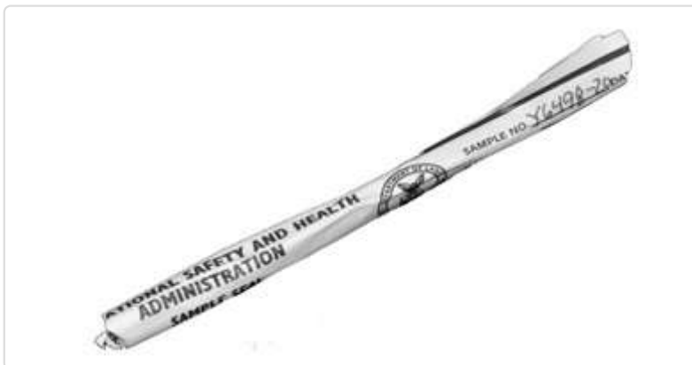
Figure G-1. Correctly Sealed Charcoal Tube. Charcoal Tube Inside Form OSHA-21
