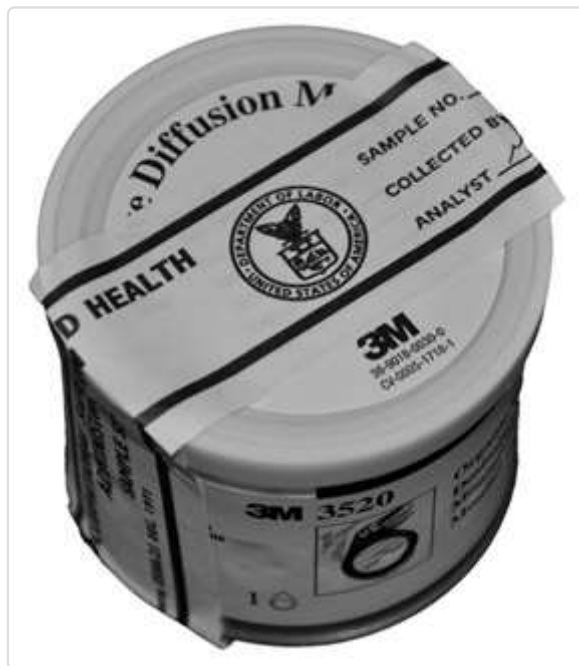
Correctly sealed 3M passive monitor
