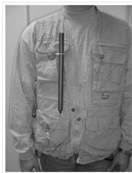
Figure 5. Large Protective Tube Cover for Sorbent Tubes in Series (Photo courtesy of NIOSH)
