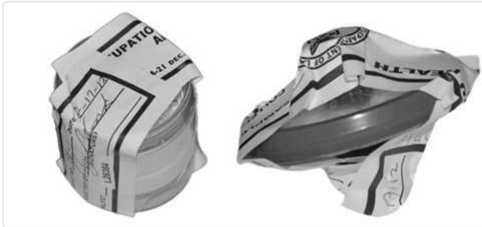
Figure G-4. Correctly Sealed Cassette With Form OSHA-21 Covering Inlet/Outlet Ports Maintaining Sample Integrity
