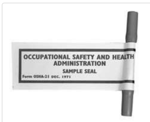
Figure G-2. Incorrectly Sealed Charcoal Tube. End Caps Can Be Removed, Allowing Sample Integrity To Be Jeopardized Without Disturbing the Seal
