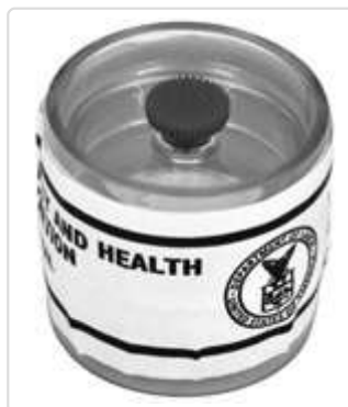
Figure G-3. Incorrectly Sealed Cassette Allows Access to Inlet/Outlet Ports After Sample Has Been Taken
