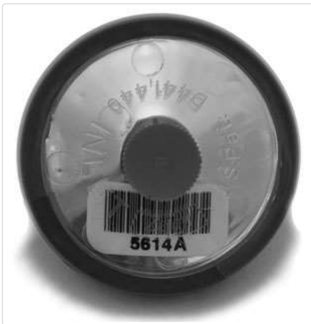
Figure A-4. Inlet View of a Filter Cassette (open to atmosphere, pointed downward during sampling)
